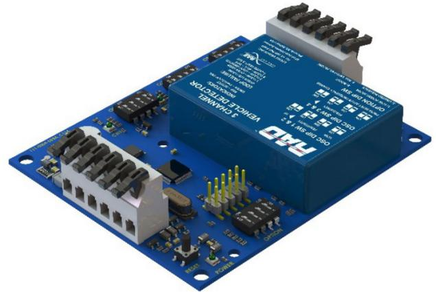
**Controls:** Board mounted DIP switches on the top of the board allow the user to set up frequency & sensitivity for each channel. Another four position Dip switch (Option switches) at the bottom of the board will set up Low Power, Boost, Limited Presence, and Fail-Safe or Fail-Secure operation.
