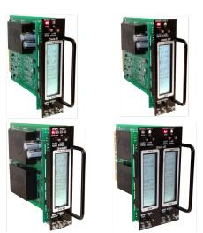
**LCD View Screens:** The Loop Frequency,  $-\Delta L/L\%$ , Loop Inductance, DEFLECTOMETER® Pie Graph, DEFLECTOMETER® Numeric Optimizer, DEFLECTOMETER® Streaming Graph, Frequency Stability Graph, Sensitivity Level, Mode of Operation, and Vehicle Counting Accumulator can be viewed on the front panel LCD for each channel simultaneously.
