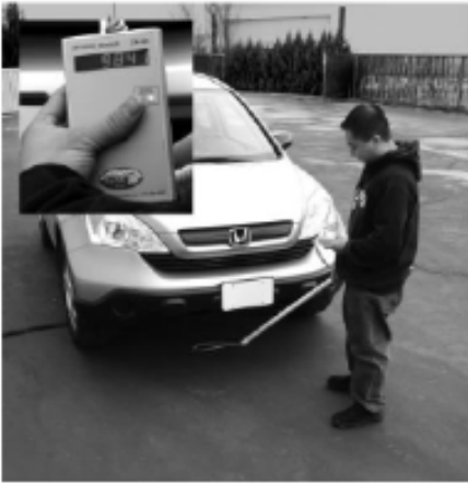
Figure 4. Reading AVI code transmitted from AVI-ATT using AVI code reader. (Code 9841 being read.)
