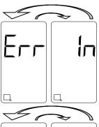
Internal EEPROM Error. The display will toggle between the two screens shown with a 50% duty cycle. This is an indication that the data stored on the internal EEPROM is corrupt. Press the FUNC pushbutton to copy the reference data stored on the external EEPROM memory module to the internal EEPROM. If the error message does not clear, the internal EEPROM is defective. Return the detector to the factory for servicing.
