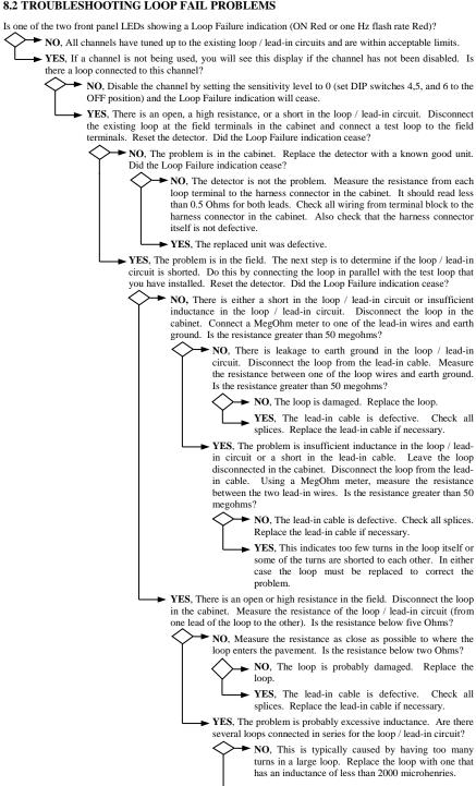
→ YES, If possible, connecting each loop to its own detector is preferred. Or try a parallel wiring arrangement for the loops if separate detection channels are not possible.
