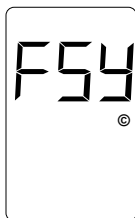
Series Synch Mode Failure Indication
