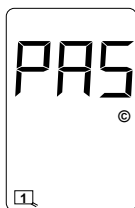
Loop Check Pass Indication
