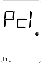
Loop Check Pending Indication
