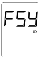
Parallel Synch Mode Failure Indication
