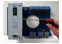
Step 4: Remove the front panel / PC board assembly from the detector housing.
