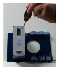
Step 3: Insert the end of the small, flat bladed screwdriver between the front panel and the detector hosing. Carefully twist the screwdriver to pry the front panel away from the detector housing. To avoid damaging the detector PC board, do not insert the screwdriver more than 0.125 inch.
