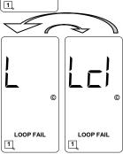
If the check loop verification process continues for the entire 55 second period and no action has been taken to connect or restore the check loops causing the check loop verification, the LCD screen will toggle between the two screens shown with a 50% duty cycle.
