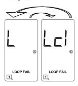
Loop Check Failure Indication
