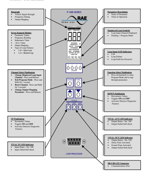
NOTES: The LCD backlighting illuminates whenever any pushbutton is pressed. Backlighting will extinguish 15 minutes after the last pushbutton press.
