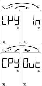
Parameters stored on the motherboard mounted EEPROM do not match those stored on the internal EEPROM. Pressing the FUNC pushbutton will accept the parameters stored on the internal EEPROM and store them on the motherboard mounted EEPROM, i.e. copy the internal EEPROM parameters to the motherboard mounted EEPROM.
