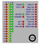
The indicator for a field input will be on if the RMS voltage over the last 33 milliseconds (two cycles of AC power) is above the threshold for that type of input. (See Section 3.2 for the voltage levels for each type of input.)
