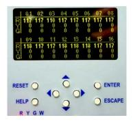
Down Pushbutton – The pushbutton labeled ▼ is used to navigate through menu selections or settings being viewed. Pressing this pushbutton while at the bottom of a menu will advance the cursor to the first menu item. If the setting being viewed can be changed, and the setting is displayed on a line consisting of more than one entry, pressing this pushbutton will decrement the setting. When at the Run Time Display, this button will decrease the front panel LED dimming level.
