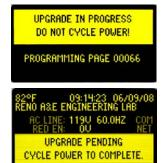
Each firmware file is encrypted and contains information identifying what model monitor it can be used in and what type of firmware it is. This ensures that the user cannot inadvertently upgrade a monitor with the incorrect firmware and that the firmware file has not been tampered with.
