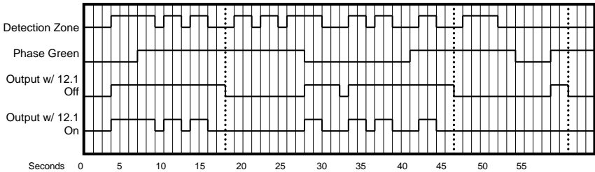
This example assumes an extension time of 2 seconds. The dotted lines show where disconnect would occur. Phase Green is the state of the light (actual Phase Green Input is inverted).
