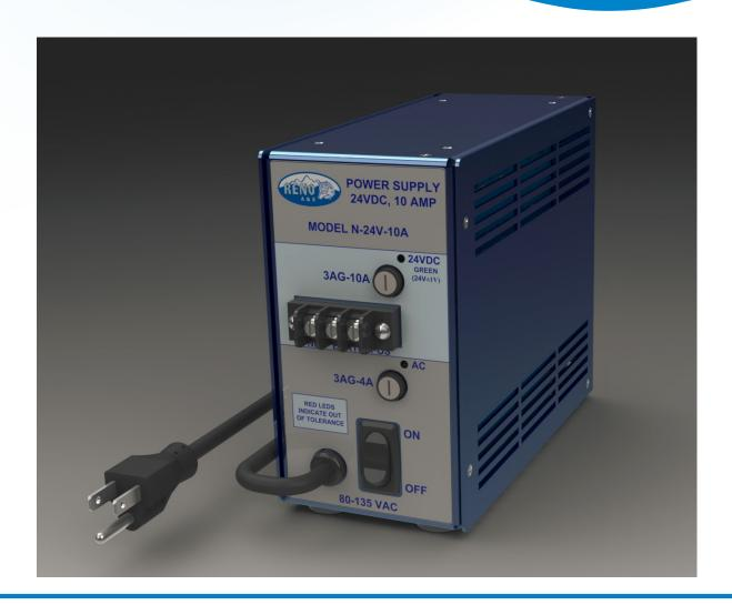
Models: N-12V-10A, N-13V-10A, N-24V-10A Input: 80 VAC to 135 VAC, 45-65 Hz Outputs\*: 12VDC, 13VDC, 24VDC @ 10Amps \*Contact Reno A&E for other output voltages
