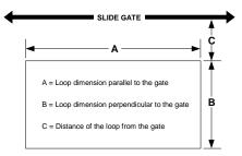
1 Mark the loop layout on the pavement. Remove sharp inside corners that can damage the loop wire insulation.
