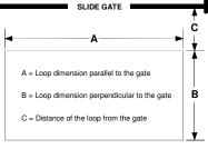
For reliable detection of small motorcycles, legs A and B should not exceed 6 feet.
