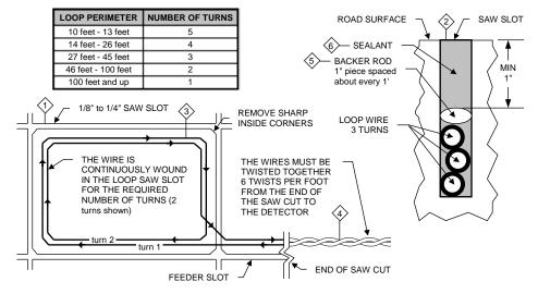
Recommended Loop Wire: Reno LW-120 for 1/8" slots Reno LW-116-S for 1/4" slots
