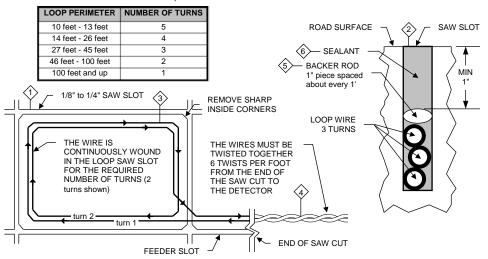
Recommended Loop Wire: Reno LW-120 for 1/8" slots Reno LW-116-S for 1/4" slots
