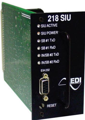
The SIU-218 Serial Interface Unit (SIU) performs the interface between Serial Bus #1 of the Advanced Traffic Controller (ATC) and the Input Assembly, Output Assembly, and other devices in an ITS modular cabinet assembly. Its functions include controlling load switch outputs, detector resets, communicating with inductive loop detectors and other devices, and the conditioning and conversion of loop detector inputs for the ATC.
