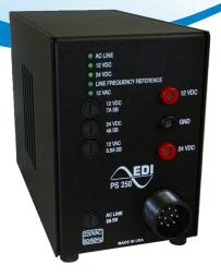
A separate LED indicator is provided to display output status and fuse integrity for the two DC supply outputs (12VDC, 24VDC) and the 12 Vac output (12VAC). The Line Frequency Reference indicator pulses to show 50/60 Hz activity. An indicator is also provided for the AC Line input (POWER).
