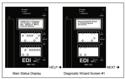
The first step of the Diagnostic Wizard provides a simple definition of the fault type detected. It also filters the Channel Status display to a concise view of only the channels actually involved in the fault.
