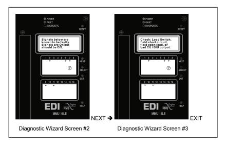
In Type 16 mode, the next steps pinpoint known faulty signals. Type 12 operation does not have the benefit of Field Checking (screen #2) unless the *Type 12 with SDLC* mode (Section 1.4.2.1) is selected, so the MMU2-16LE *SmartMonitor* does not have enough information to actually identify the faulty signals. The last step offers the technician several suggestions for the cause of the malfunction.
