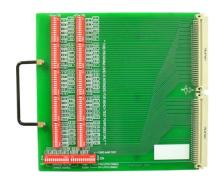
The MMU-EXT Program Card is designed to facilitate cabinet testing when multiple Program Card configurations are needed. DIP switches for all programmable functions of the MMU Program Card make modifications to the MMU set-up fast and easy.
