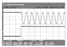
Repeat the above for the second loop detector channel. If the above waveform is not found on one or both channels of the detector, possible fault areas are Q8 (Q9), Q11 (Q13), Q7-A (Q7-B), CR13 (CR14), or T1 (T2).
