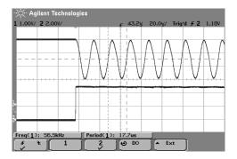
Repeat the above for the second loop detector channel. If the above waveform is not found on one or both channels of the detector, possible fault areas are Q8 (Q9), Q11 (Q13), Q7-A (Q7-B), CR13 (CR14), or T1 (T2).
