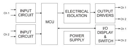
The MCU then controls the OUTPUT and DISPLAY blocks appropriately. The TEST switches can be used to force the input to the True state. If the TEST switch is in the ON (locked) or MOM (momentary) position it will force the output to the asserted (True) state regardless of the input circuit state. The TEST switches are processed through the MCU for pulse width input and output requirements.
