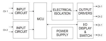
The MCU then controls the OUTPUT and DISPLAY blocks appropriately. If jumper SEL3 or E3 is installed a valid input pulse will generate an output pulse of 100 milliseconds minimum.
