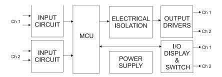
The MCU then controls the OUTPUT and DISPLAY blocks appropriately. If jumper SEL3 is installed a valid input pulse will generate an output pulse of 100 milliseconds minimum.
