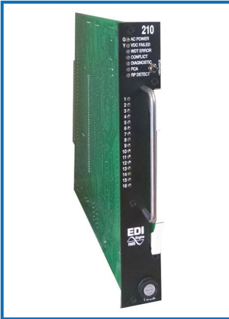
The EDI 210 Series Signal Monitor is designed to provide the basic monitoring requirements for Caltrans Type 170 Output Files. The unit is fully compatible with the requirements of the Model 170 Controller Unit.
