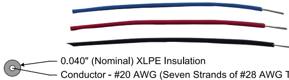
Conductor - #20 AWG (Seven Strands of #28 AWG Tinned Copper Wire)
