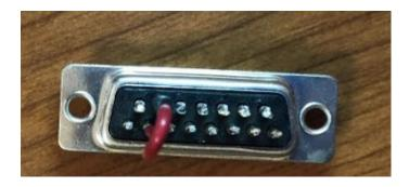
Once you have completed step 3, put the DB15 into the **PORT 1 SDLC** of the monitor and reset the monitor. The **Port 1 Fail** and **Fault LED** will clear.
