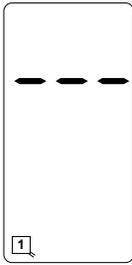
If the detector passes its check loop verification process or a pending loop check failure state is resolved in one of the ways mentioned above, the LCD screen will show a normal (idle) condition.
