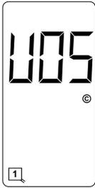
Upon application of power, the LCD screen will show the detector model letter and firmware version, in this case, Model U-1400 firmware version 5. This screen will be displayed for two seconds.
