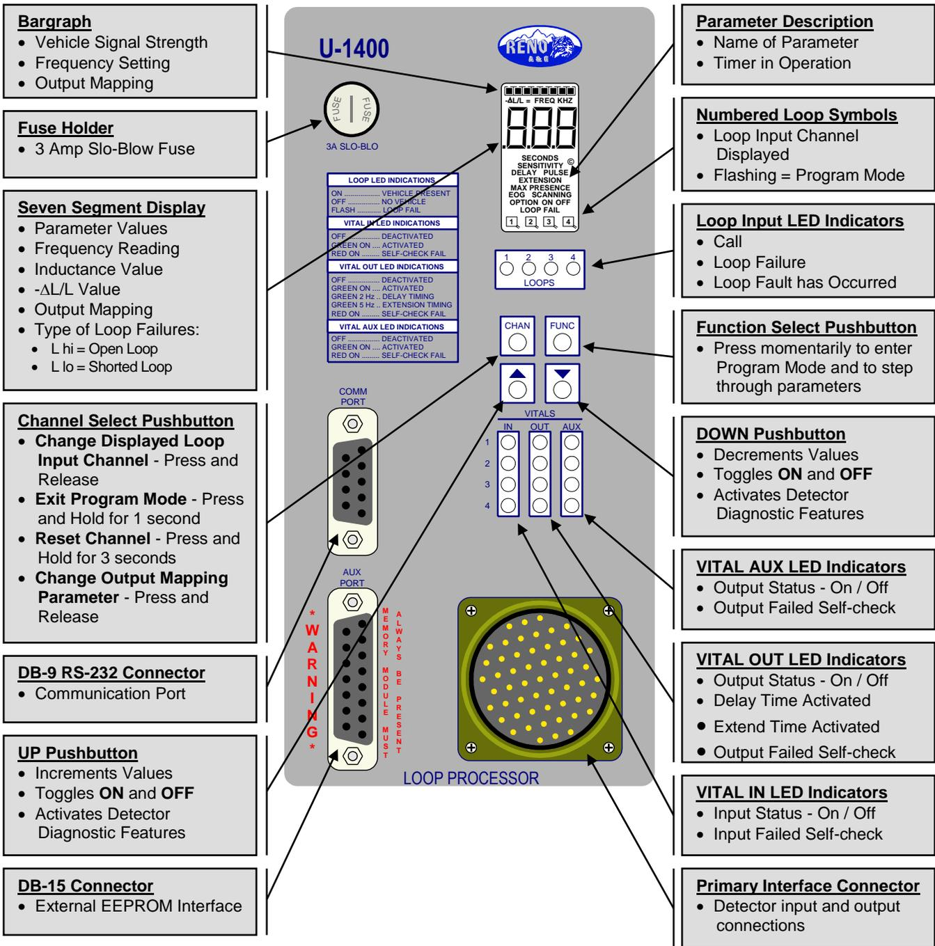
NOTES: The LCD backlighting illuminates whenever any pushbutton is pressed. Backlighting will extinguish 15 minutes after the last pushbutton press.
