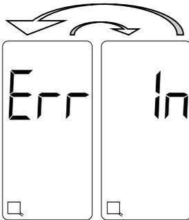
**Internal EEPROM Error.** The display will toggle between the two screens shown with a 50% duty cycle. This is an indication that the data stored on the internal EEPROM is corrupt. Press the **FUNC** pushbutton to copy the reference data stored on the external EEPROM memory module to the internal EEPROM. If the error message does not clear, the internal EEPROM is defective. Return the detector to the factory for servicing.
