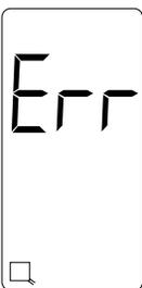
**Detection Reference Error.** This is an indication that the internal EEPROM and the external EEPROM memory module detection reference values do not match. Press the **FUNC** pushbutton to clear the error message.
