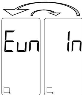
**Uninitialized Internal EEPROM.** The display will toggle between the two screens shown with a 50% duty cycle. This is an indication that the internal EEPROM is uninitialized. To correct this problem, press the **FUNC** pushbutton. If the error message does not clear, the internal EEPROM is defective. Return the detector to the factory for servicing.
