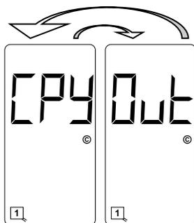
Parameters stored on the external EEPROM memory module do not match those stored on the internal EEPROM. Pressing the **FUNC** pushbutton will accept the parameters stored on the external EEPROM memory module and store them on the internal EEPROM, i.e. copy the external EEPROM memory module parameters to the internal EEPROM.
