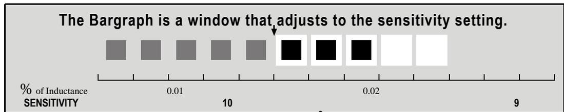
The bargraph below has the same vehicle in the loop zone causing the same inductance change as above. Because the sensitivity setting was increased to Level 8, six segments are now displayed. If the bargraph displays 5 or 6 segments for a vehicle in the loop, the sensitivity has been set to the proper range.
