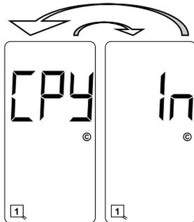
Parameters stored on the external EEPROM memory module do not match those stored on the internal EEPROM. Pressing the **FUNC** pushbutton will accept the parameters stored on the internal EEPROM and store them on the external EEPROM memory module, i.e. copy the internal EEPROM parameters to the external EEPROM memory module.
