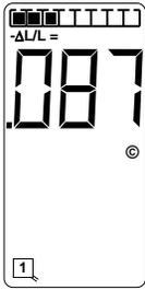
**STATE** ..... Loop Inductance - $\Delta L/L$  Display (% Change) (Option 2 ON).
