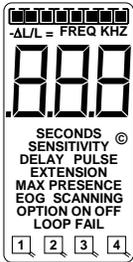
**STATE** ..... LCD Display Test.
