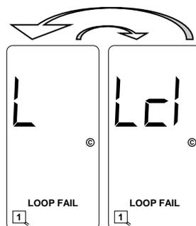
If the check loop verification process continues for the entire 55 second period and no action has been taken to connect or restore the check loops causing the check loop verification, the LCD screen will toggle between the two screens shown with a 50% duty cycle.
