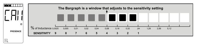
The bargraph, below, has the same vehicle in the loop zone causing the same inductance change as above. Since the sensitivity setting was increased to Level 7, six segments are now displayed. If the bargraph displays 5 or 6 segments for a vehicle in the loop and motorcycles are not a concern, the sensitivity has been set to the proper range.
