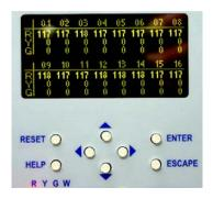
Down Pushbutton – The pushbutton labeled ▼ is used to navigate through menu selections or settings being viewed. Pressing this pushbutton while at the bottom of a menu will advance the cursor to the first menu item. If the setting being viewed can be changed, and the setting is displayed on a line consisting of more than one entry, pressing this pushbutton will decrement the setting. When at the Run Time Display, this button will decrease the front panel LED dimming level.
