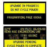
Each firmware file is encrypted and contains information identifying what model monitor it can be used in and what type of firmware it is. This ensures that the user cannot inadvertently upgrade a monitor with the incorrect firmware and that the firmware file has not been tampered with.
