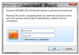
The configuration settings of the monitor Ethernet port can be password protected using the *Authentication* page, Section 4.8.).
