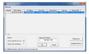
Once a monitor has identified itself, the network configuration parameters may be modified if necessary by right clicking on the table entry or selecting the *Configure Device* button. This provides a mechanism for configuring the IP address, subnet mask, and default gateway of the monitor port. Note that the network parameters are accepted only in decimal notation; hex and octal digits are not allowed.
