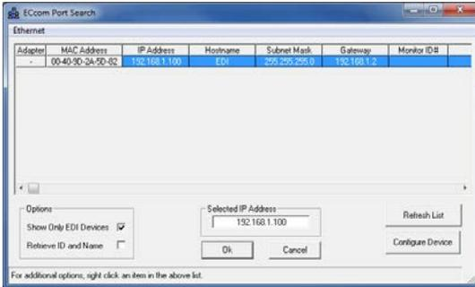
Once a monitor has identified itself, the network configuration parameters may be modified if necessary by right clicking on the table entry. This provides a mechanism for configuring the IP address, subnet mask, and default gateway of the monitor port. Note that the network parameters are accepted only in decimal notation; hex and octal digits are not allowed. Depending on the Ethernet port version of the monitor one of the following windows will be displayed.
