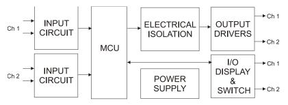
The MCU then controls the OUTPUT and DISPLAY blocks appropriately. If jumper SEL3 is installed a valid input pulse will generate an output pulse of 100 milliseconds minimum.
